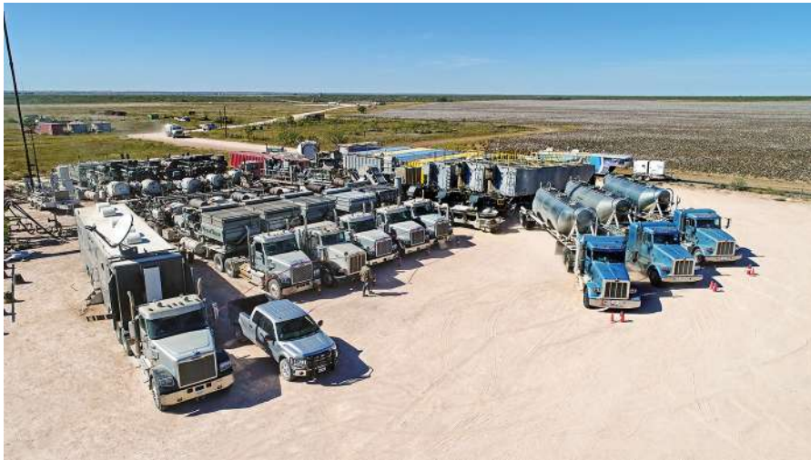
Fig. 4. Service providers can't simply bring in raw reservoir gas to fuel dual-fuel frac fleets. Even where sufficient reservoir gas is available, the supply must be tested—and frequently treated—on location, to ensure that it is suitable to use.
