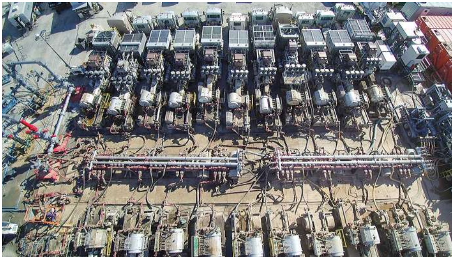
Fig. 4. Service providers can't simply bring in raw reservoir gas to fuel dual-fuel frac fleets. Even where sufficient reservoir gas is available, the supply must be tested—and frequently treated—on location, to ensure that it is suitable to use.
