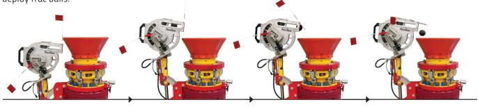
As shown in the above simulation, the RBD sits safely out of the way of the lubricator when disengaged. Then, when the operator remotely engages the hydraulic controls, the unit provides a safe, reliable ball drop.
