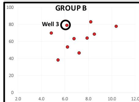
Cross-plot for each group with six-month production ( $\text{BOE} \times 10^3$ ) on Y axis and total proppant volume ( $\text{lbs} \times 10^6$ ) on X axis
